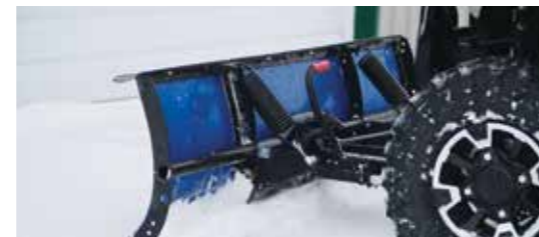
BACK DRAG MODE ALLOWS FOR PULLING SNOW AWAY FROM BUILDINGS
