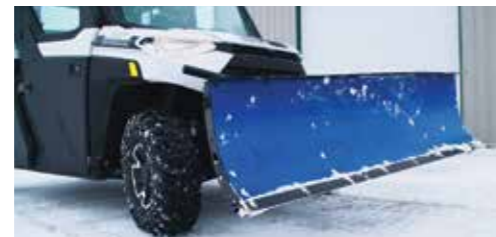
PLOW IS AUTOMATICALLY RAISED WHEN SHIFTING INTO REVERSE
